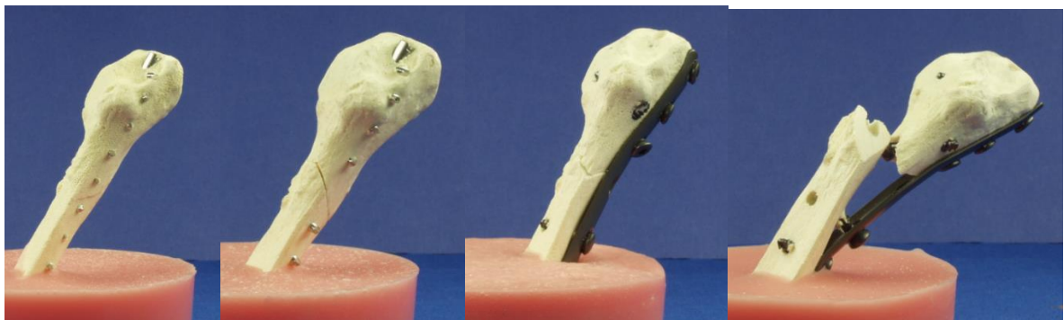
Fig.166 XS-nail has a much higher resistance to axial compression than the locked plate, wich diforms and leads to damage of the fixation assmbly.
